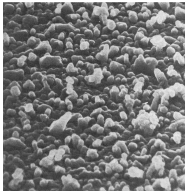
Figure 2 —Scanning electron micrograph of the coating of stearic acid formed on a potassium chloride disk by sublimation of stearic acid ( \times 1900 ).
